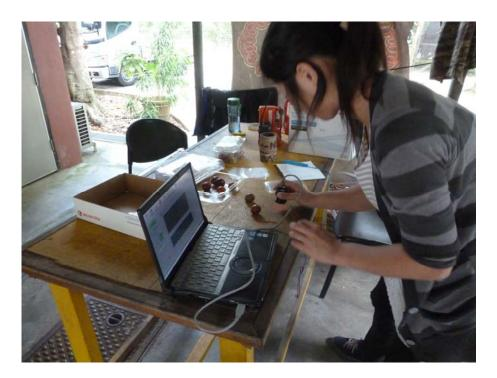
Fig. Scanning prune fruits by NIR spectrometer
