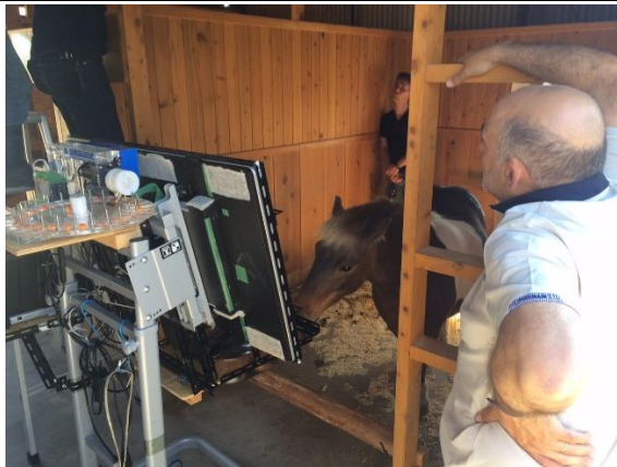
Universal feeder, computer and touch screen.
