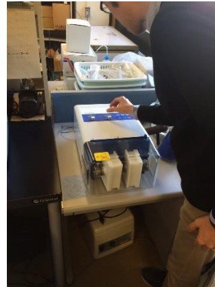
A ‘TissueLyser’ grinding up our sporophyte samples
